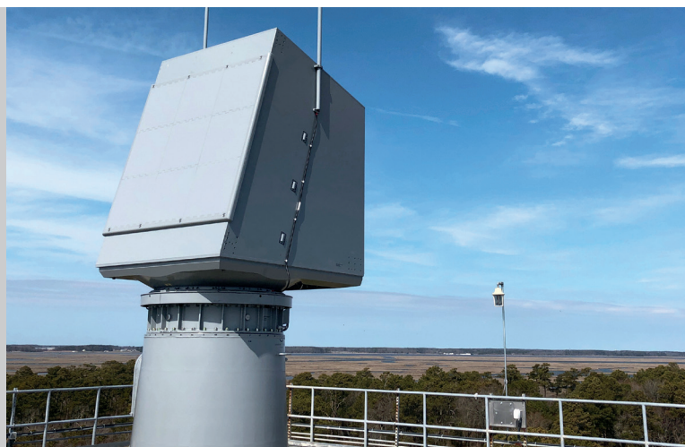
▲ Tactical radars like Raytheon Missiles & Defense's SPY-6(V)3 will benefit from concepts developed in the Network Cooperative Radar program.
